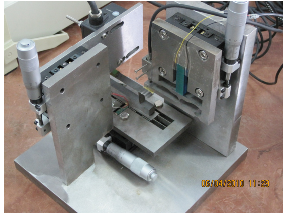
Fig. 21. Prototype of designed indentation device
