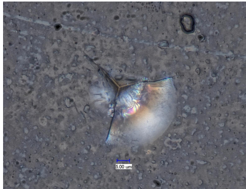
Fig. 37. Indentation morphology of optical glass
